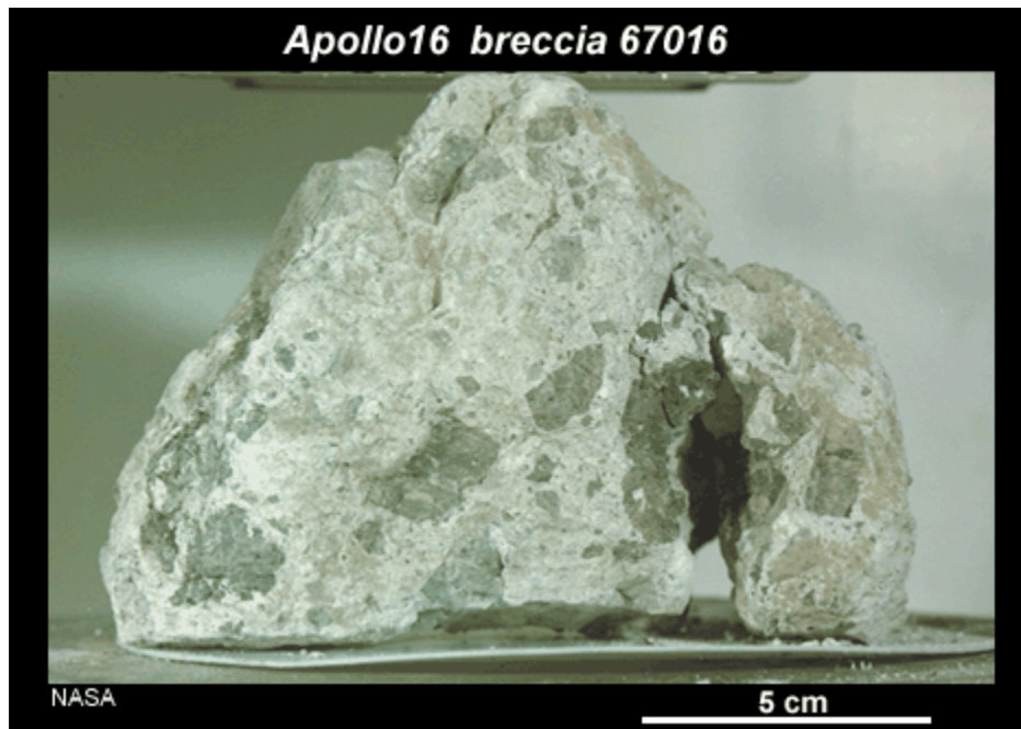
67016 is an impact breccia that was collected from the rim of North Ray crater, Apollo 16. It consists of fragments of plagioclase (white) and glass (dark gray). Rock fragments in breccias like these tell us a great deal about the early history of the Moon.
