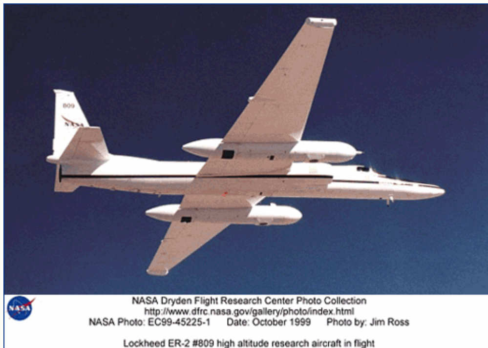
ER-2 airplane in flight. Ultra-clean dust collectors are mounted under the wings (not shown in this view).
