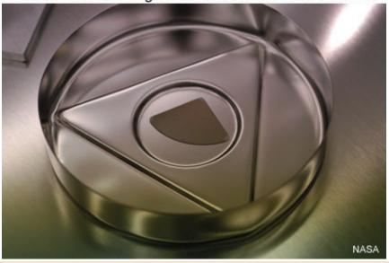
Portion of the high-purity SiC collector from the solar wind concentrator returned by the Genesis Mission. Samples are stored and handled in a special laboratory at NASA Johnson Space Center.
