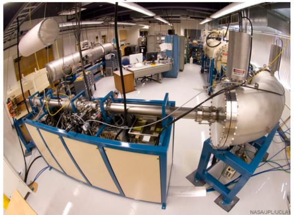
The MegaSIMS is a hybrid instrument consisting of a secondary ion mass spectrometer (Cameca ims 6f) front-end combined with an accelerator mass spectrometer, whose purpose is to eliminate molecular interferences via dissociation. See the labeled schematic diagram for names of parts shown in the photos.
