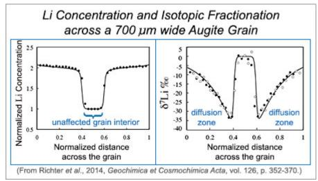
Experimental results of the diffusion of lithium into an *augite* grain. [LEFT] Lithium concentration is normalized to 1 in the grain interior. The data points show an abrupt step in concentration toward the grain interior. [RIGHT] Richter and coauthors found lithium isotopic fractionations of <sup>7</sup>Li/<sup>6</sup>Li of about 30‰ in the diffusion zones. The lines in both figures are profiles calculated using a diffusion model, described by Richter and coauthors in their paper.
