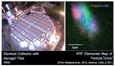
**[LEFT]** The Stardust Interstellar Dust Collector is composed of two sides of aerogel tiles set in aluminum framing. One side collected dust from Comet Wild 2 and the other side collected particles as the spacecraft flew through the interstellar dust stream. **[RIGHT]** Elemental map derived from X-ray fluorescence data of one of the candidate interstellar dust particles, named Orion, found in aerogel.
