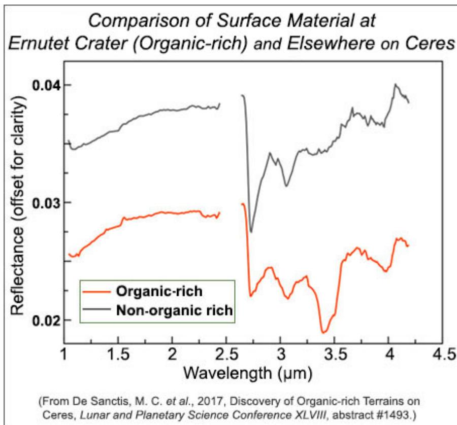
Spectra from the visible and infrared imaging spectrometer on board the Dawn spacecraft at the Ernutet crater region on Ceres. The red line: spectrum of organic-rich material near the crater rim, which shows the distinctive 3.3–3.5  $\mu\text{m}$  absorption band. The gray line: spectrum of non-organic-rich material in an area several kilometers eastward from Ernutet crater. (Source: LPSC XLVIII abstract #1493.)
