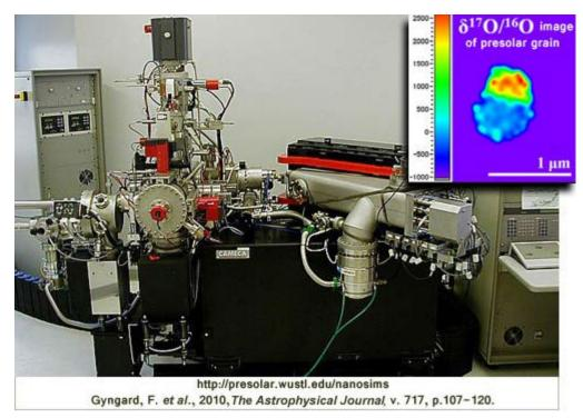
Development of high-tech instruments make it possible to analyze the abundances of isotopes in these astonishingly small grains. The NanoSIMS at Washington University in St. Louis, MO is one such workhorse. Gyngard and coauthors developed an automated, high-massresolution measurement technique for the NanoSIMS to analyze thousands of grains over several days without requiring a scientist's constant attention. It differs from previous
