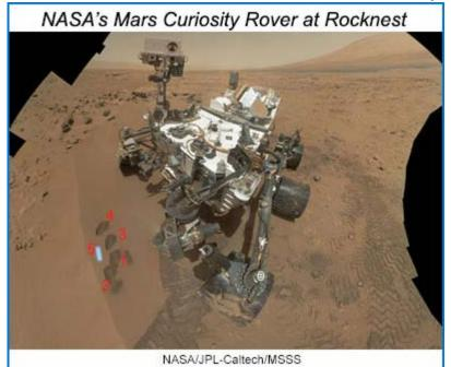
Using the rover's Alpha-Particle X-ray Spectrometer (APXS) and the CheMin powder X-ray diffraction instrument, first authors David Blake (NASA Ames Research Center) and David Bish (Indiana Univeristy) and coauthors describe the samples collected from this accumulation of windblown particles, also known as the Rocknest sand shadow.
