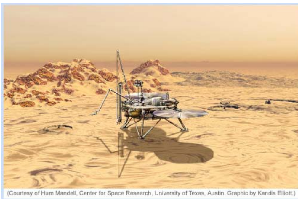
(Courtesy of Hum Mandell, Center for Space Research, University of Texas, Austin. Graphic by Kandis Elliott.) Painting of a concept for a Mars lander equipped with a drill.
