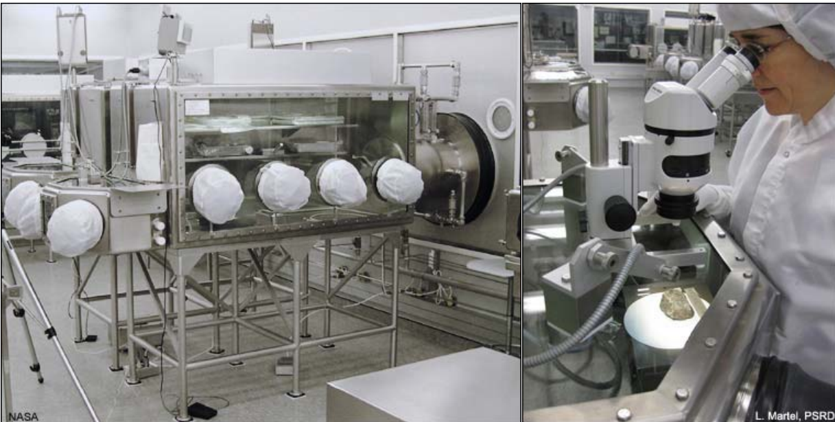
NASA is in charge of organizing and storing the Apollo lunar materials. [LEFT] Samples are transferred for processing or examination into these sealed, stainless-steel glove cabinets in the Lunar Sample Laboratory at the NASA Johnson Space Center in Houston, Texas. The cabinets are continuously purged by nitrogen, a relatively non-reactive gas, to create an environment with minimum chemical reactions with the samples. Gloves are fitted to holes in the sides of the cabinets, capped when not in use, so that workers can reach and handle the samples. The special airlock into the wall, on the right side of the cabinet, opens to the pristine corridor where the samples are transferred to and from the storage vault. [RIGHT] Here I am inside the laboratory examining an Apollo 15 lunar breccia with an optical microscope at one of the cabinet viewing stations; photo by Jeff Taylor.
