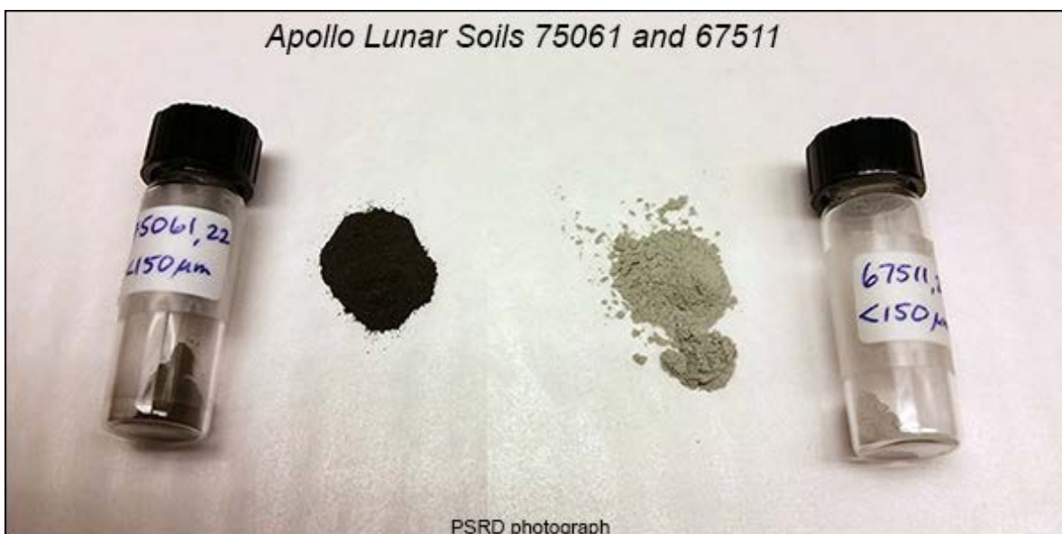
Photograph of the <150 micrometer size fraction of two lunar regolith (sometimes simply called soil) samples, one from the Apollo 16 site in the highlands (67511) and one from the Apollo 17 site in the maria (75061; the 7 is only partly visible in the photo). Each pile contains thousands of grains, essentially all of which have been exposed to the solar wind.
