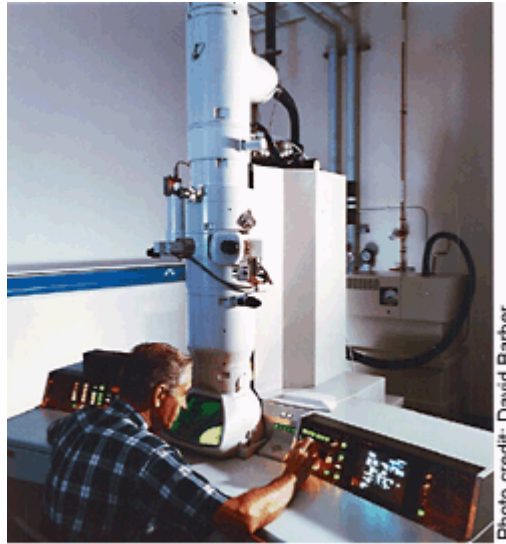
David Barber at the helm of a JEOL 2010 analytical transmission electron microscope operating at 200 kV at the Hong Kong University of Science and Technology.
