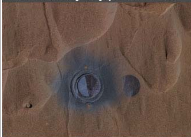
Rock "Mazatzal" after grinding by rock abrasion tool
