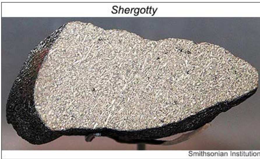
Photo of a sawn surface of the Shergotty meteorite. Large whitish grains are pyroxene. The dark surface on this stone is the fusion crust , formed during entry into the Earth's atmosphere.
