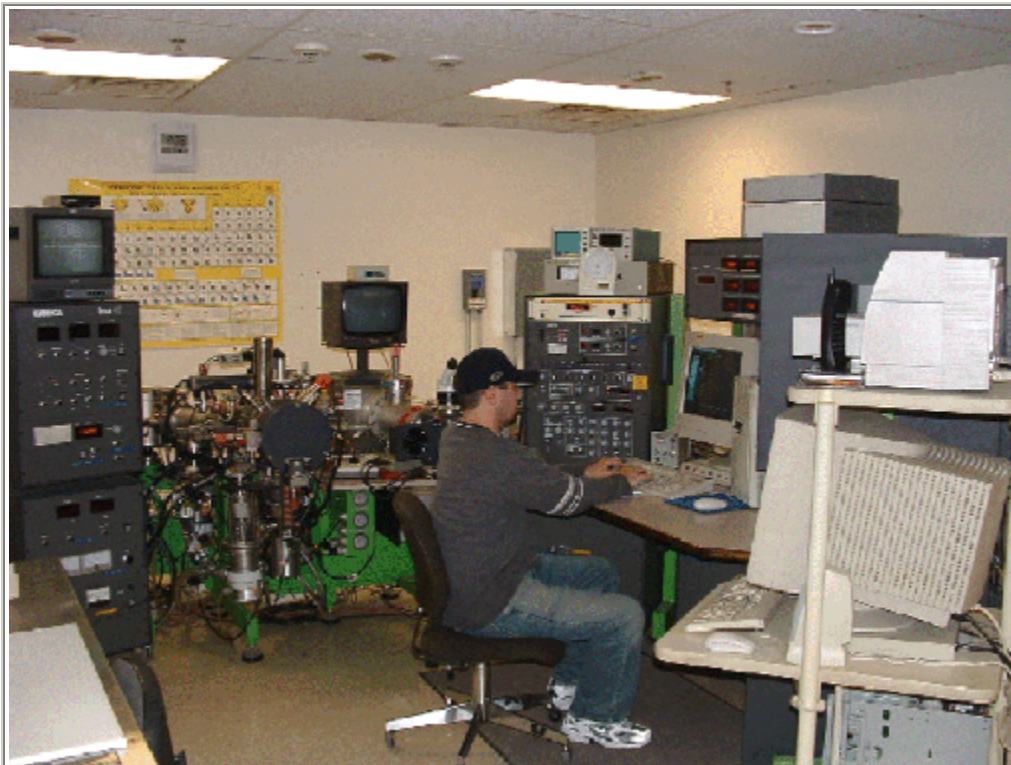
The concentrations of tungsten were measured with the ion microprobe at the University of New Mexico. This complicated instrument consists of an ion source, mass spectrometer, and associated electronics and vacuum system. Shown operating the ion probe is Justin Hagerty, a graduate student at UNM.
